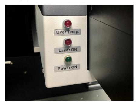
There are 3 LED lights on the panel and they will indicate out three working status of "Over Temp", "Laser On" and "Power on" of the laser marker.
