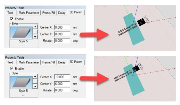
**Step 14.** After finishing all settings, please click the "Preview or button to do the dry run and make sure the marking position is correct.
